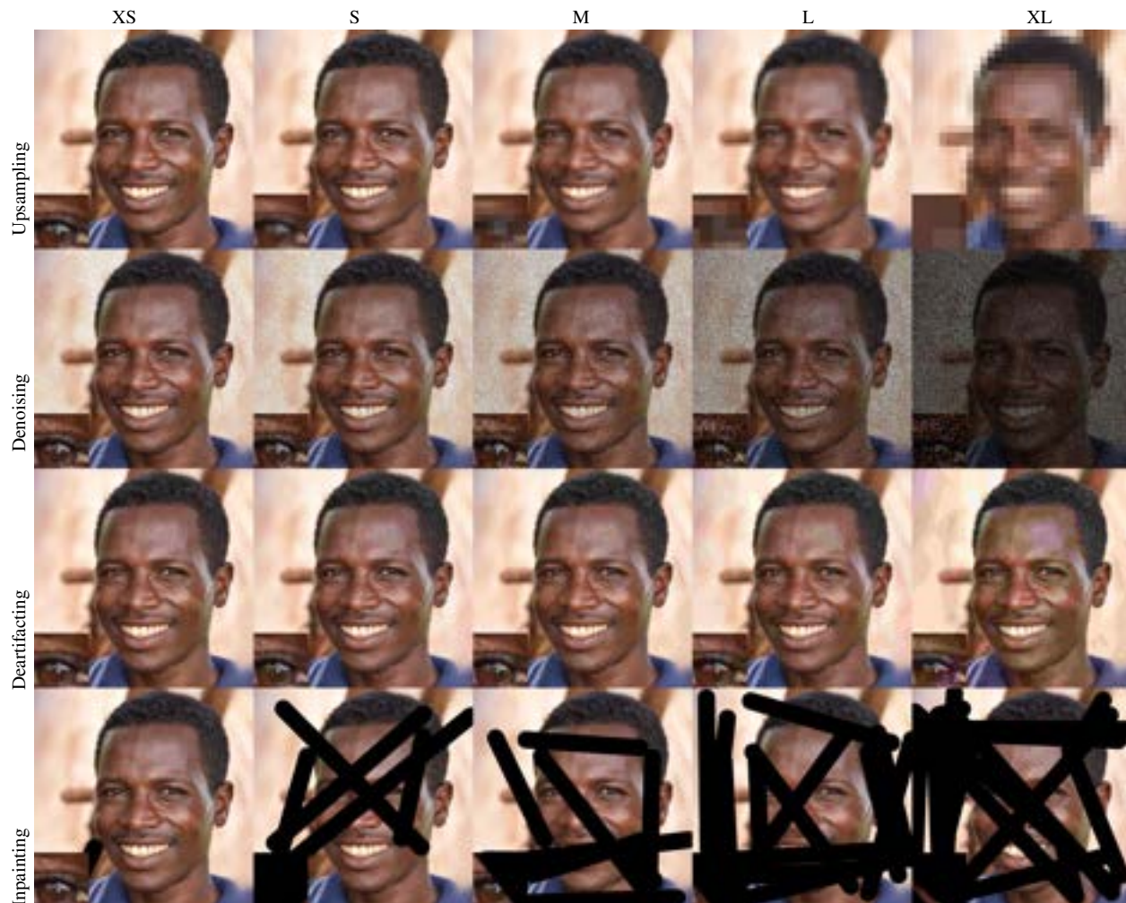
Figure 6. All degradation levels used in our benchmark (from left to right: XS, S, M, L, XL; from top to bottom: upsampling, denoising, deartifacting, and inpainting). Please note that all images have native resolution 1024 \times 1024 ; inlays (bottom-left of each image) magnify 4\times a small 32 \times 32 crop near the left eye. Please zoom in to better appreciate the levels.
